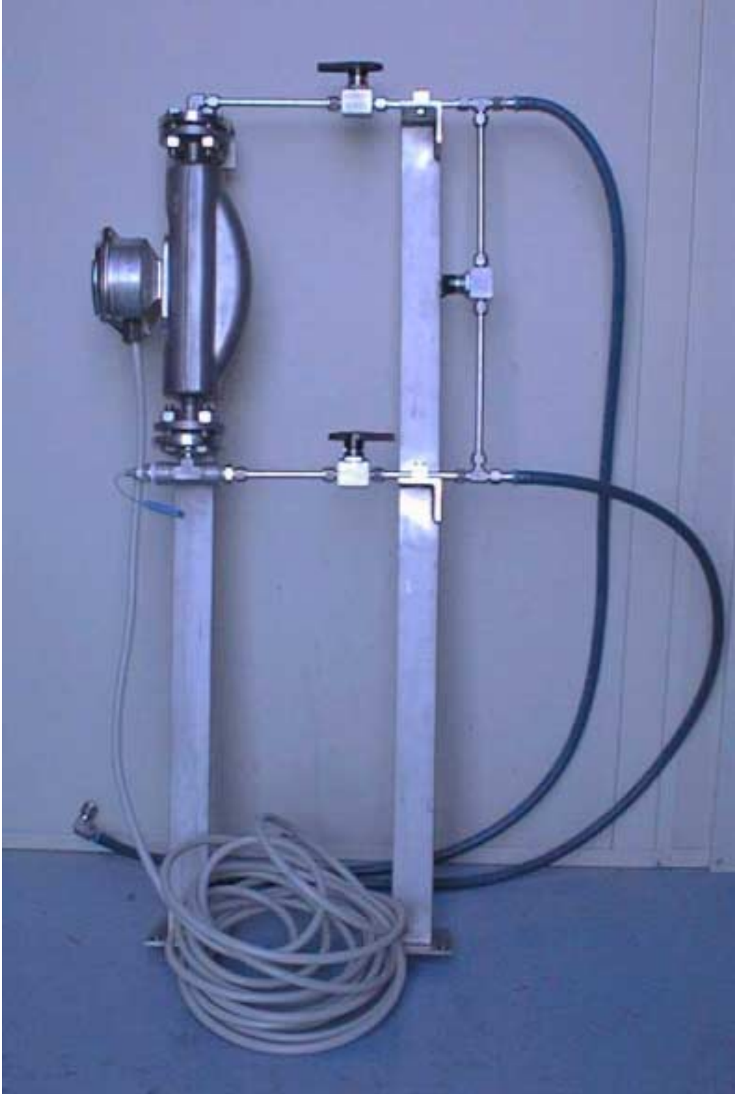
Fig. 2. Photograph of the Endress + Hauser Promass 63F Coriolis meter installed in its apparatus.
