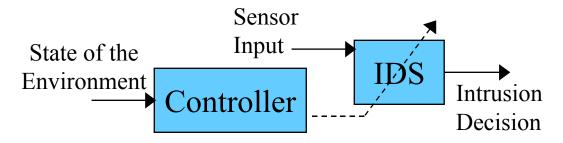
Figure 5. State-based intrusion detection system control.
