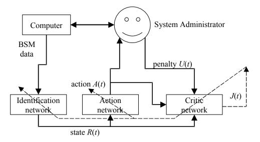
Figure 12. Adaptive critic design for BSM-based intrusion detection.
