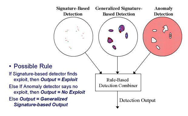
Figure 3. Potential combination of intrusion detection approaches.
