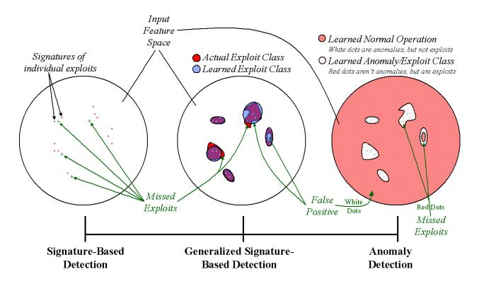
Figure 2. Comparison of different intrusion detection approaches in reality.
