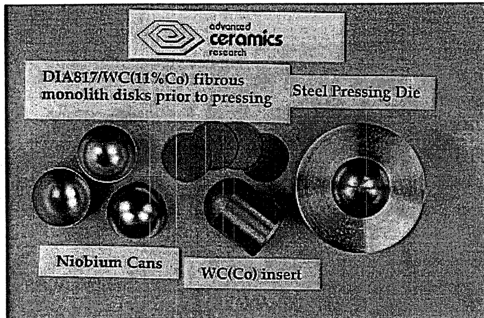
Figure 15. Photograph of DIA817/WC(11% Co) fibrous monolith green discs and the lamination tooling used to press and shape the discs.
