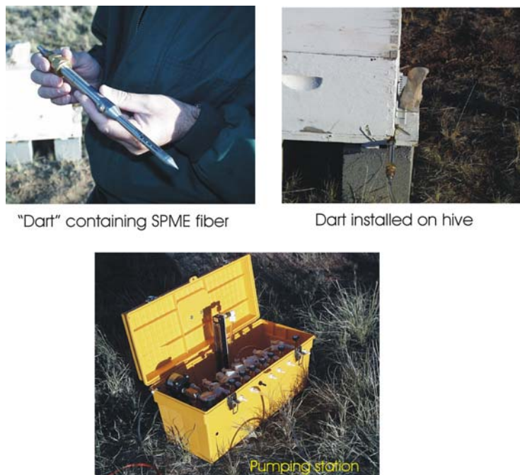
Figure 3: Photos of test configuration.
