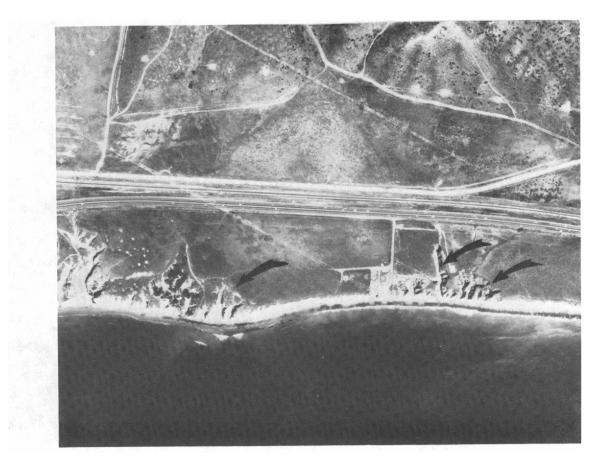
Figure 59. Vertical aerial view of the coastal terrace in 1953 at the present site of the San Onofre Nuclear Power Plant. Arrows point to Barranca-gully development along and into coastal terrace (photograph by U.S. Department of Agriculture).
