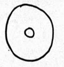
To compute f in terms of h and A, we simulate a lattice cell by an "equivalent cylinder". Within the graphite of this cylinder
