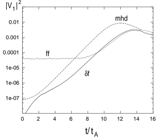
*Fig.5: The temporal evolution in the  $n = 1$  component of kinetic energy from MHD,  $\delta f$  hybrid and full  $f$  hybrid simulations all done for the same equilibrium profiles with  $E = 3.9$  and  $\bar{s} = 7.4$ .*
