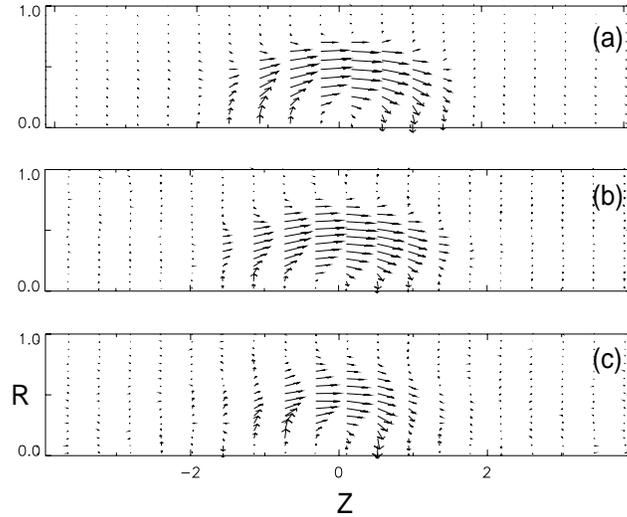
*Fig.8: Vector plots of poloidal component ( $r - z$  plane) of the ion fluid velocity: (a) from the MHD simulation, (b) and (c) from the hybrid simulations with  $\bar{s} = 7.4$  and  $\bar{s} = 0.9$ ,  $E = 3.9$ .*
