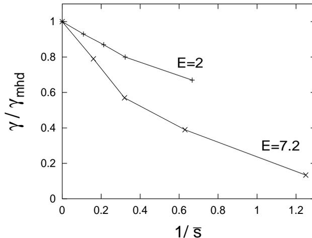
*Fig. 7: Variation of the normalized growth rate of the  $n = 1$  tilt instability with  $1/\bar{s}$  parameter. The points obtained in the linearized hybrid simulations for two different elongations,  $E \approx 2$  and  $E = 7.2$ , are indicated.*
