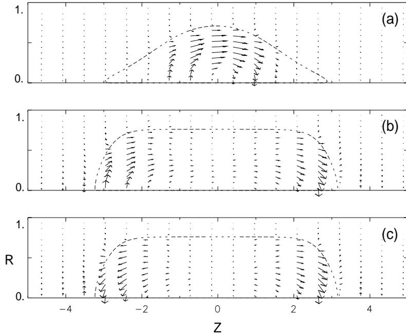
*Fig.1: Velocity vectors and the separatrix positions from MHD simulation of the  $n = 1$  tilt mode ( $E = 4$ ); (a) elliptical separatrix, (b) racetrack separatrix, and (c)  $n = 1$  even mode with the racetrack separatrix.*
