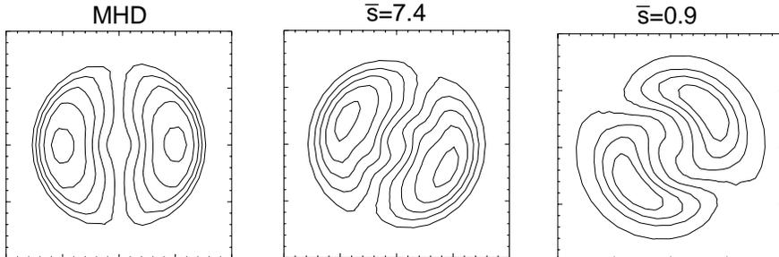
*Fig.9: Contour plots of the axial component (at the midplane) of the ion fluid velocity: (a) from the MHD simulation, (b) and (c) from the hybrid simulations with  $\bar{s} = 7.4$  and  $\bar{s} = 0.9$ , same simulations as on Fig.8.*
