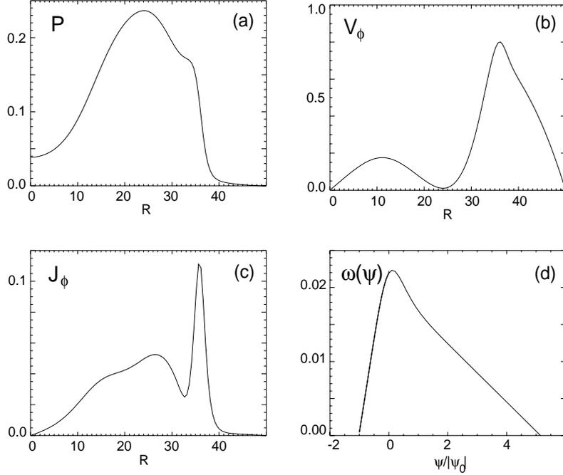
*Fig.3: The equilibrium profiles for MHD simulations with sheared rotation: the radial profiles of (a) plasma pressure, (b) toroidal velocity and (c) current at the midplane, and (d) angular rotation velocity versus normalized flux for the equilibrium with  $E = 2.7$  and  $M_s = V_s/V_A = 0.8$ .*
