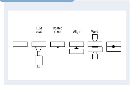
The kinetic energy metallization (KEM) process can be used to effect two types of bonding for aluminum and aluminum alloys.
