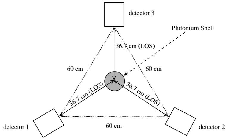
Figure 6: Top view of Pu Shell Inside Tetrahedron of Detectors
