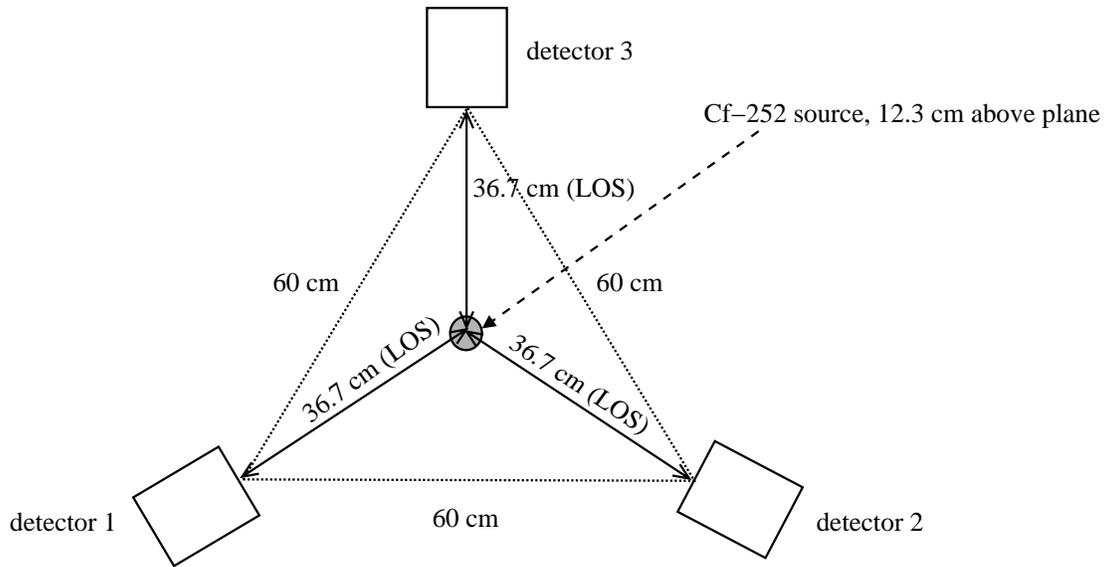
Figure 4: Top view of  $^{252}\text{Cf}$  Source and Detectors, (Det #4 not shown)
