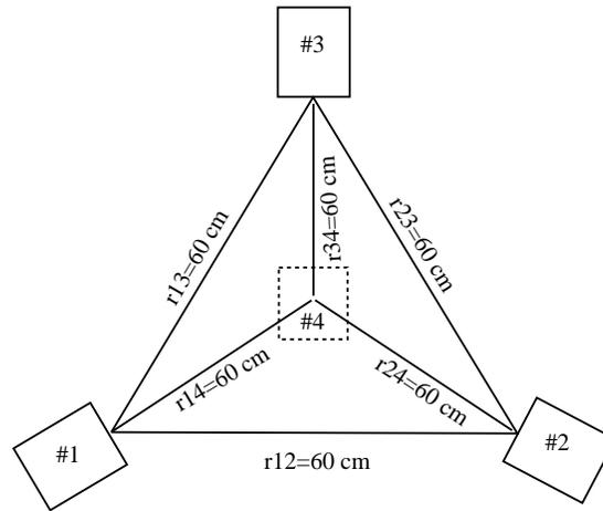
Figure 1: Top View of 4 Detectors in a Tetrahedron
