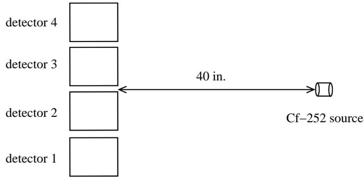
Figure 2: Time-of-Flight Setup
