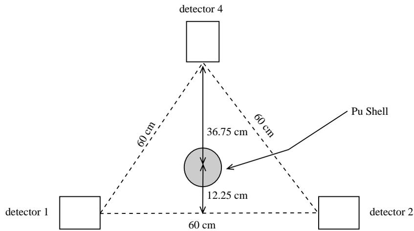
Figure 7: Side view of Pu Shell Inside Tetrahedron of Detectors
