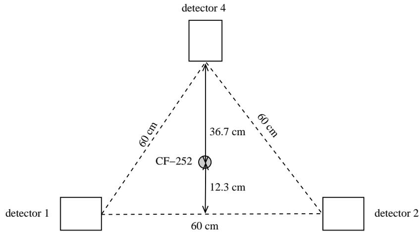
Figure 5: Side view of  $^{252}\text{Cf}$  Source and Detectors
