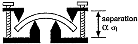
Figure 1. Schematic illustration of the concentric ring bending device used to apply stress (either tensile or compressive) to the interconnect films during a nanoindentation measurement. Note that the applied curvature is greatly exaggerated.
