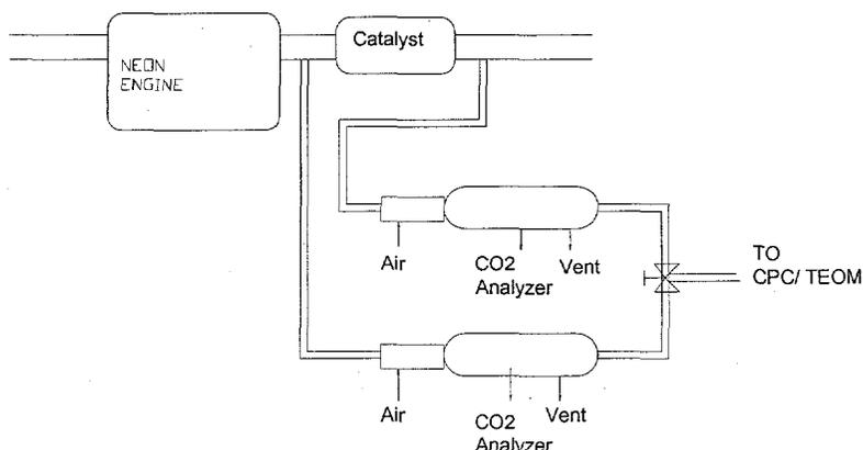
Fig. 1. A schematic of the exhaust sampling system.
