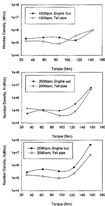
Fig. 6. Engine-out and tailpipe particulate number densities at various engine-operating conditions
