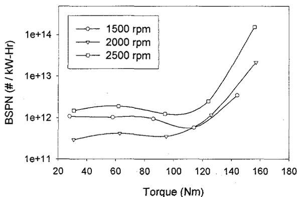
Fig. 7. Engine-out brake-specific particle number (BSPN) for various engine-operating conditions
