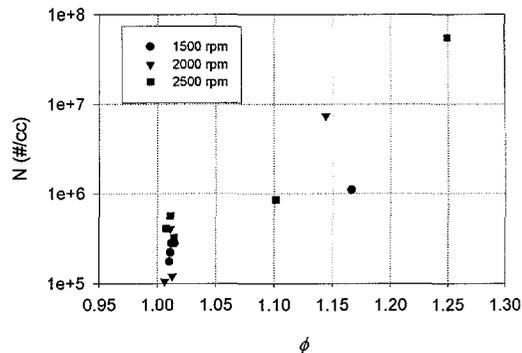
Fig. 5. Engine-out number density as a function of equivalence ratio
