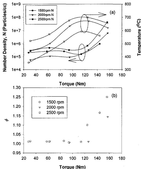
Fig. 4. Engine-out particulate number densities and exhaust temperatures at various engine-operating conditions
