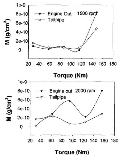
Fig. 8. Engine-out mass concentrations at various engine-operating conditions
