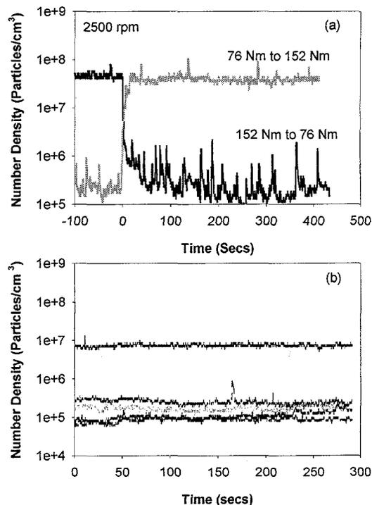
Fig. 3. (a) Transient nature of particulate emissions from an SI engine. Black - Number Density during a step transition from almost full load to half load at 2500 rpm. Grey - Number Density during a step transition from half load to almost full load at 2500 rpm. (b) Number density traces under various steady-state engine operating conditions.
