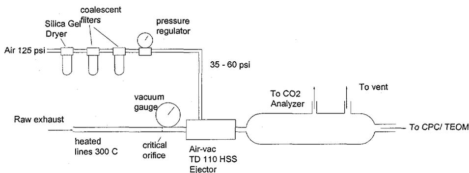
Fig. 2. Schematic of the ejector based dilution system
