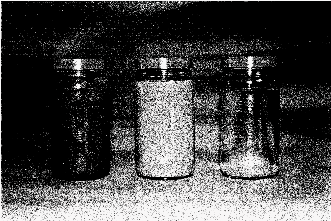
Fig. 3-1. Biosolids feed and SCWO effluent
