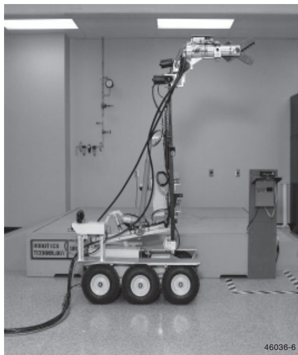
Figure 1. Mobile teleoperator used to remove a wall-mounted junction box
