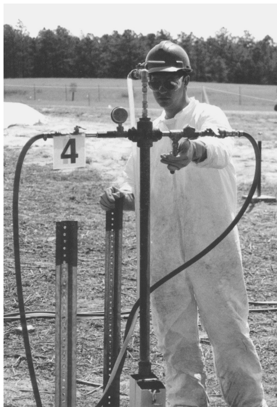
Figure 4. Fenton's Reagent is added to a source zone to destroy NAPL in place. This project was a cooperation between SRTC and industry.
