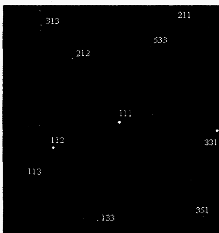
Figure 5. Laue pattern from the single aluminum grain shown in figure 4 with the silicon Laue pattern digitally subtracted.
