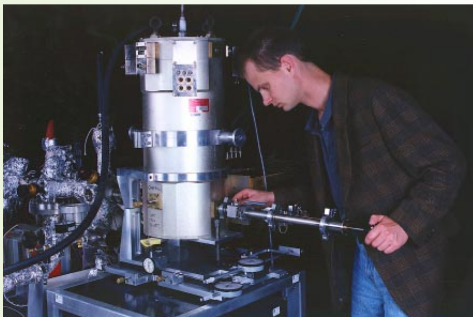
Stephan Friedrich inserts a sample in the Lawrence Livermore superconducting-tunnel-junction (STJ) detector cryostat at the Stanford Synchrotron Radiation Laboratory. X rays from the synchrotron enter the cryostat through the beamline on the left and strike the sample, producing x-ray fluorescence, which is measured by the STJ detector.
