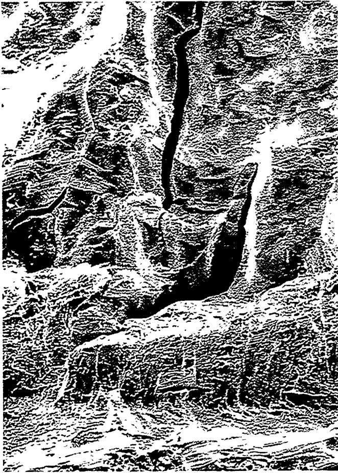
Figure 11. SEM fractograph of as-notched EN82H specimen tested in 54°C water showing ductile tearing between the base of the notch (bottom) and intergranular cracking region (upper half).
