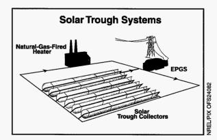
On sunny days, oil in the receiver tubes collects the concentrated solar energy as heat, and on cloudy days it is heated with natural gas. The hot oil is then pumped to an electric power generation system (EPGS) where the heat energy is converted to electricity.
