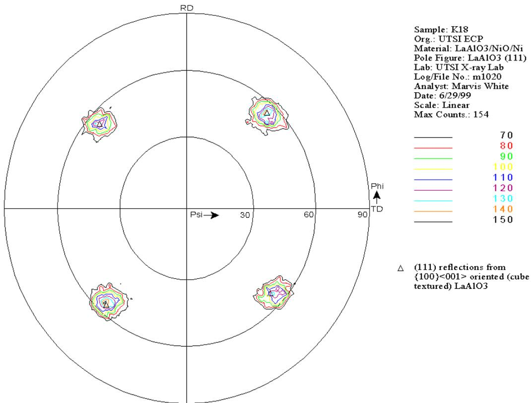
Figure 6.02-1. LaAlO<sub>3</sub> (111) Pole Figure of a Typical NiO/Ni Sample with a LaAlO<sub>3</sub> Coating on Top. No 45° In-plane Rotated Component Exist
