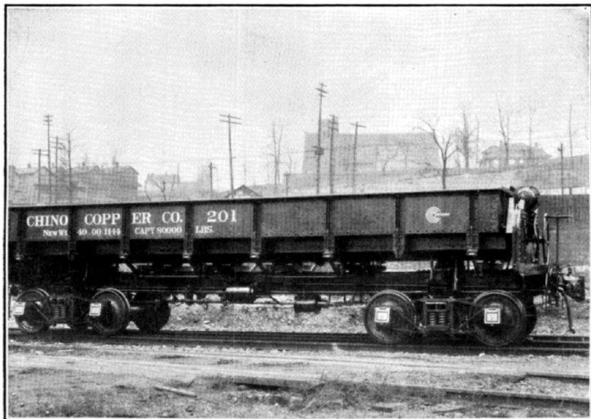
A. STEEL ORE CAR USED AT SANTA RITA. DUMPS ON EITHER SIDE BY AUTOMATIC AIR CONTROL OR BY HAND, CAPACITY 20 CUBIC YARDS.
