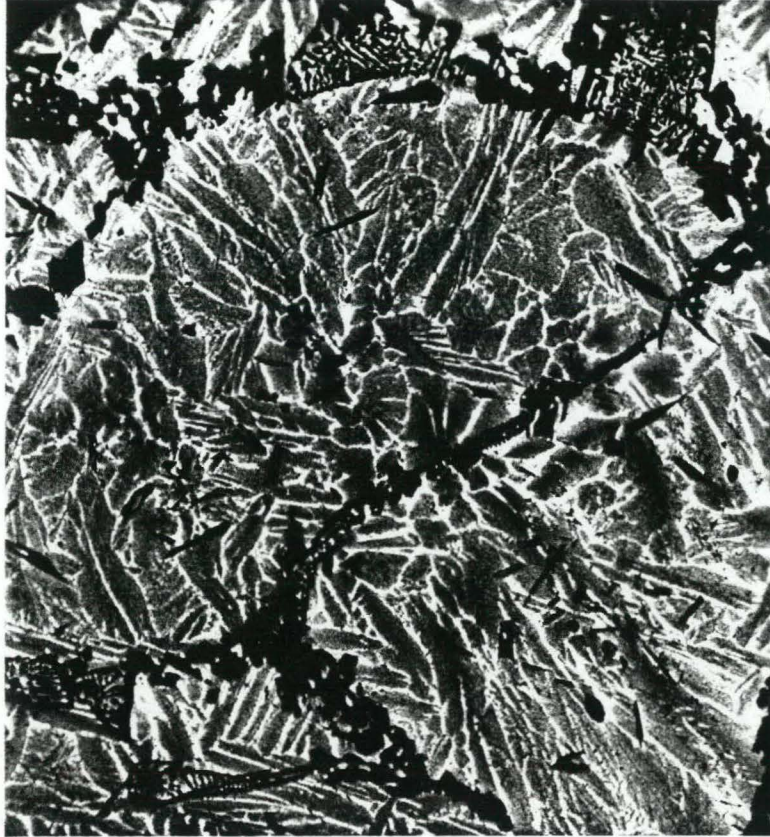
Fig. 2. Backscattered Electron Image of Zr-8SS Alloy Containing 10 wt % Pu; the Zr Solution Phase Contains some Pu, but the Bright Features Indicate High Pu Content at Phase Boundaries.
