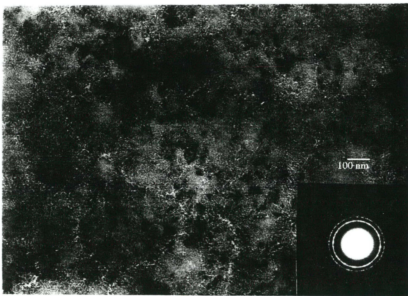
Figure 1. TEM image of a C 60 grown smooth diamond film showing the nanocrystalline structure.
