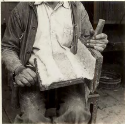
Fig. 9.--Carders with wool ready to be removed. (A) close view of cards. (B) Carder between raw wool and stack of finished slivers.
