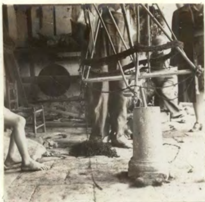
Fig. 7.--Rolling dyed yarn on shuttle-bobbins.
