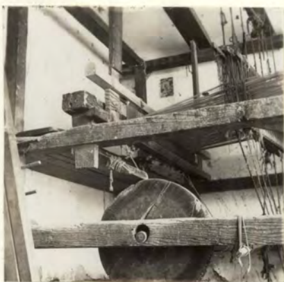
Fig. 22.--Detail from a four-heddle loom.
