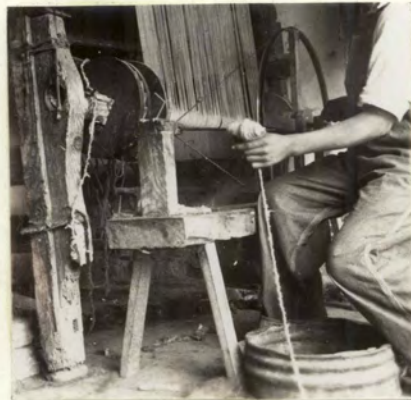
Fig. 14.--Winding spun wool on the spindle of a Jersey wheel.
