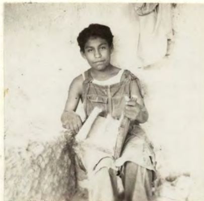
Fig. 9.--Carders with wool ready to be removed. (A) close view of cards. (B) Carder between raw wool and stack of finished slivers.
