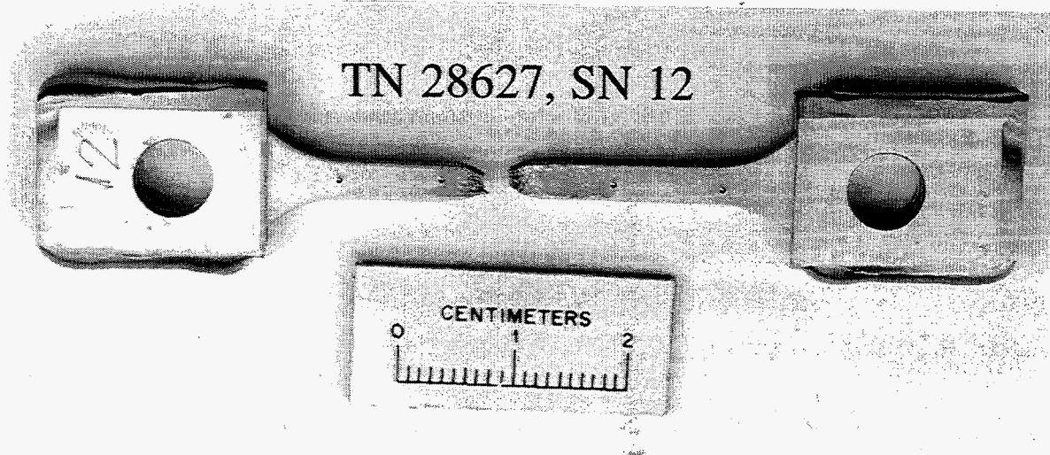
Fig. 16 After-test photographs of transverse weld samples from tests 28623 and 28627 that failed in the heat-affected zone.
