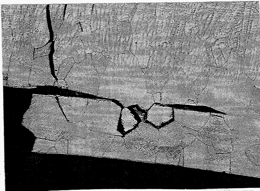
Fig. 58. Photomicrographs of a longitudinal section through the failure of capsule 15. Etched. 100 \times . (a) Outside edge and (b) inside edge (root).
