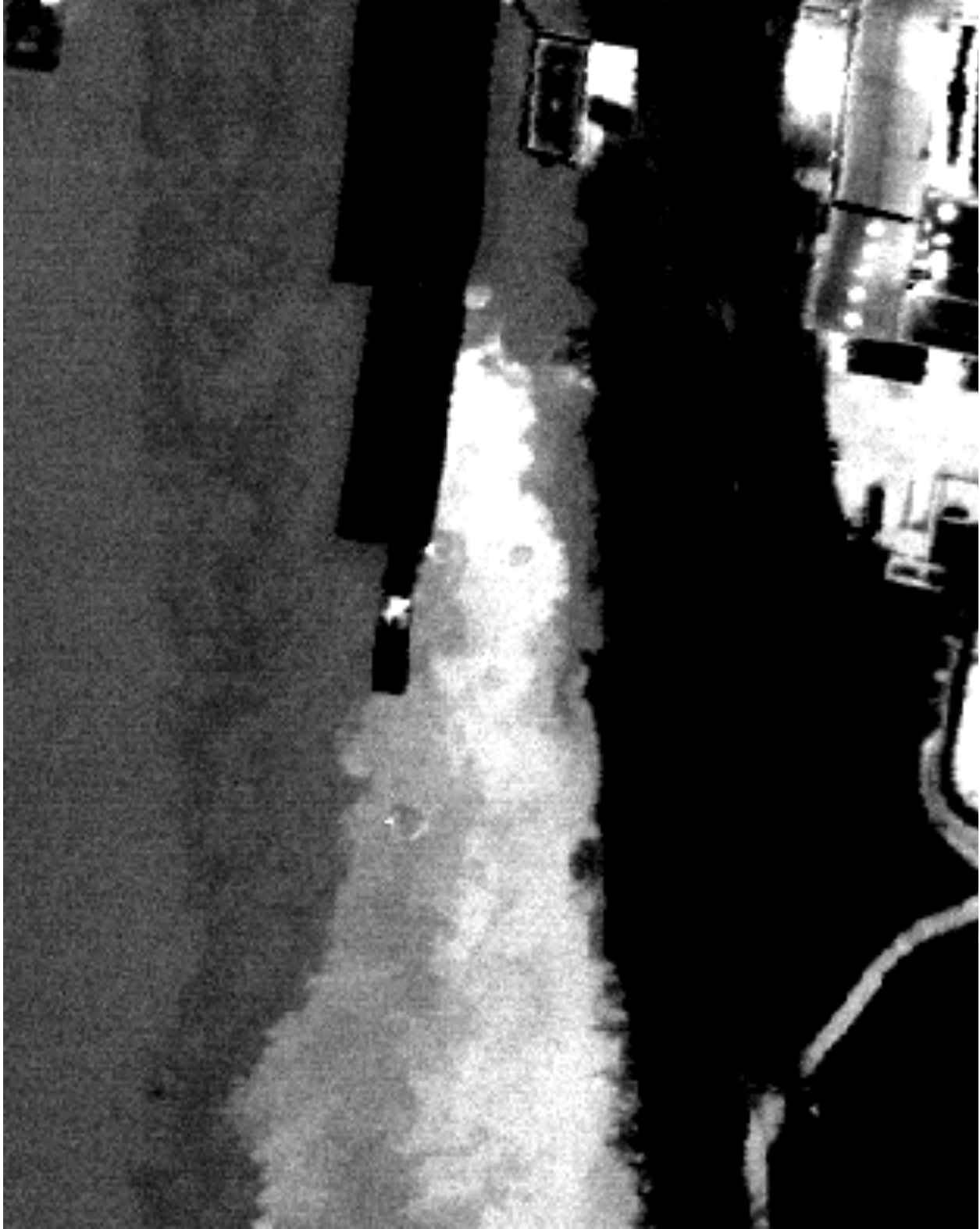
Figure 4. Example of underwater discharge from power-generating station temporarily blocked by docked coal barge. Discharge 7 degrees warmer than ambient river temperature in this instance.
