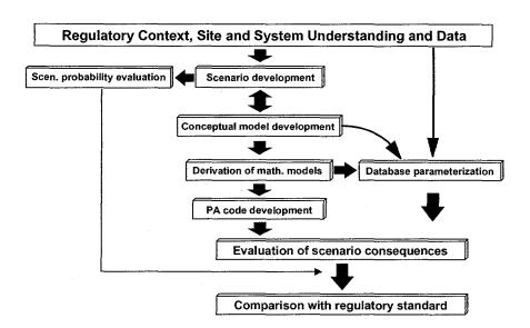
Fig. 2: Flowchart of the PA development process.
