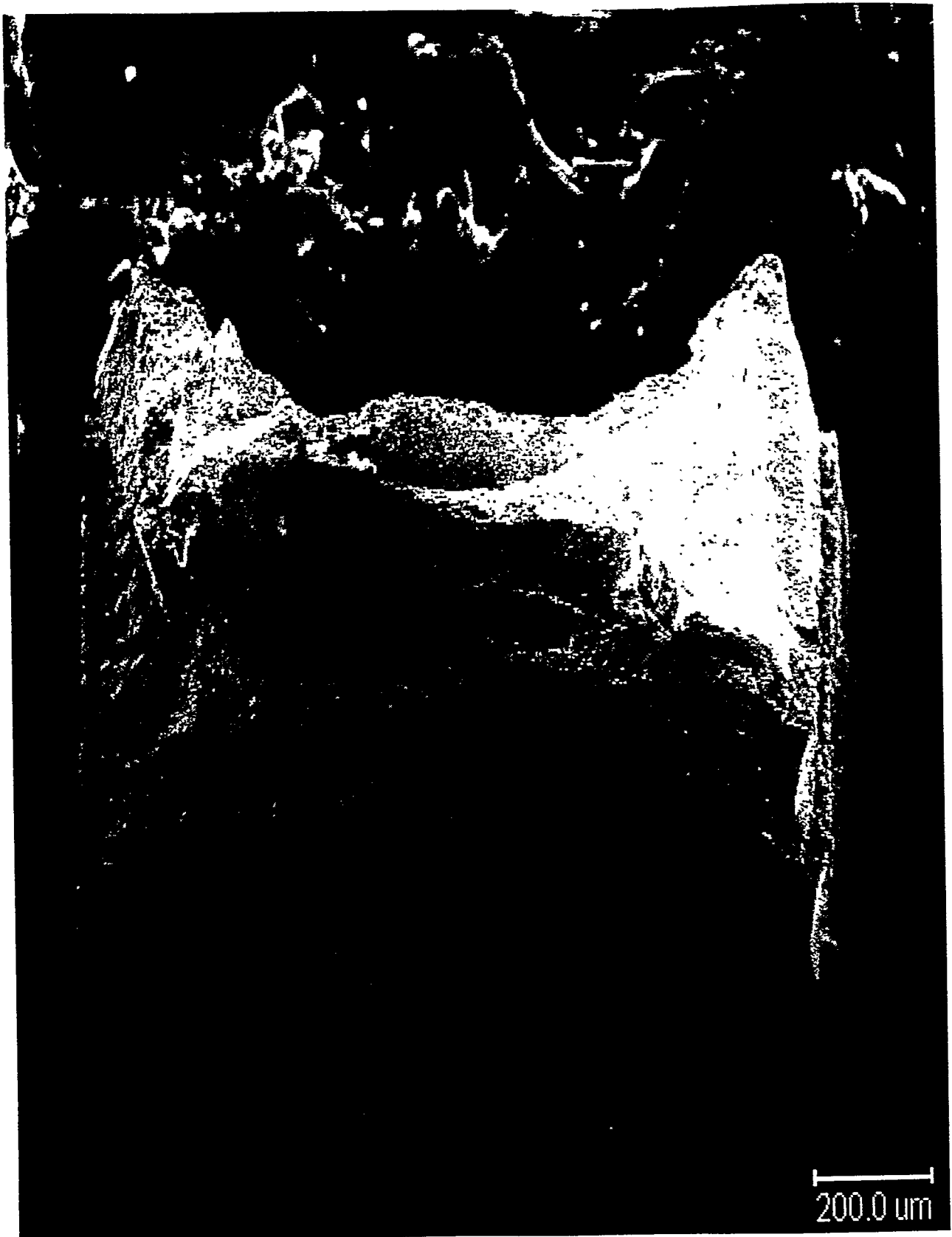
Figure 5: SEM photograph of tensile specimen 137, heat 832665, showing ductile failure (ET325901).
