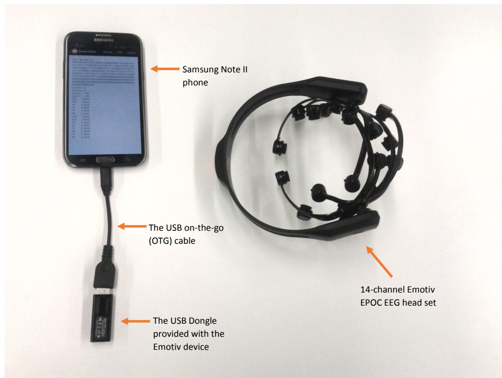
FIGURE A.9. Experimental setup to read data from the EEG headset.
