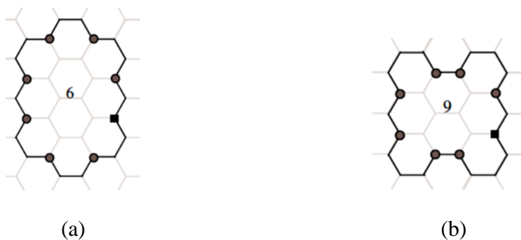
Fig. 2.9 Defects on graphene could form junction with (a) (8,0) CNT and (b) (4,4) CNT. [87]
