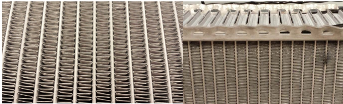
Figure 3.2: Image of radiator fin and tube configuration under investigation
