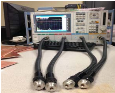
Figure 2.6. Vector Network Analyzer for the measurement of EM shielding effectiveness.
