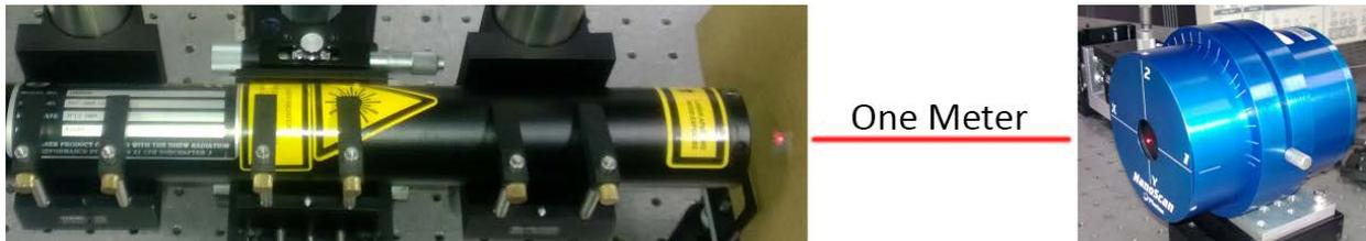
Figure 4.3 HeNe stability experiment setup
