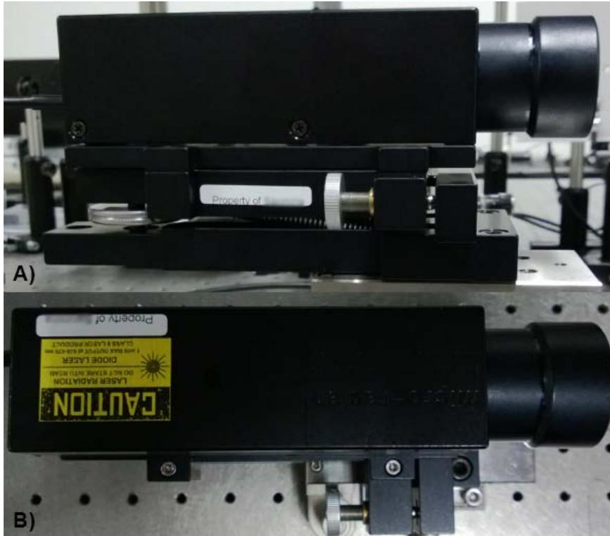
Figure 2.4 A) Side view of auto collimator and B) top view of auto collimator
