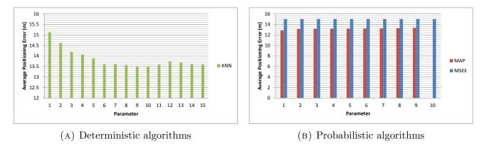
FIGURE 4.57. Average positioning error of the dynamic IPS considering 2 DAF
