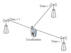
FIGURE 2.9. Calculation of position using TDOA
