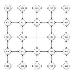
FIGURE 4.2. Ad-hoc wireless network consisting of WIFI hotspot nodes
