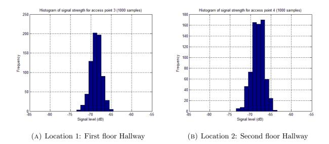
FIGURE 2.5. RSSI for 1000 samples obtained at Discovery Park
