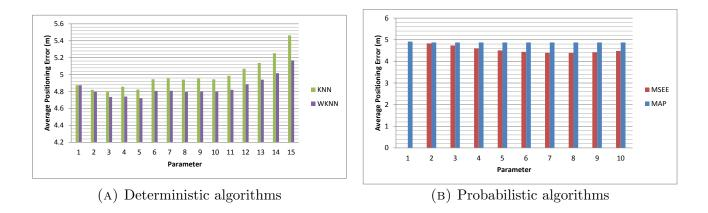
FIGURE 4.64. Average positioning error of the dynamic IPS considering 9 DAF
