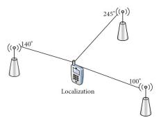
FIGURE 2.10. Calculation of position using AOA
