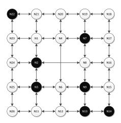
FIGURE 4.3. Combination of fixed WIFI nodes with WIFI hotspot nodes
