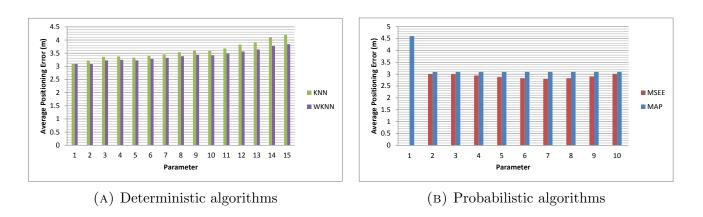
FIGURE 4.47. Average positioning error considering 2 DAF in the IPS
