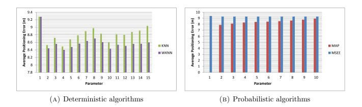
FIGURE 4.59. Average positioning error of the dynamic IPS considering 4 DAF
