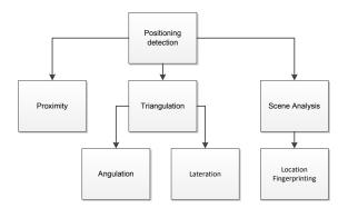
FIGURE 2.6. Classification of indoor positioning technologies and subcategories
