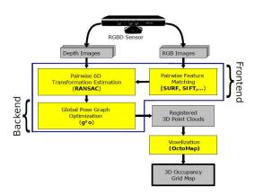
FIGURE 5.2. Schematic overview of RGBD SLAM
