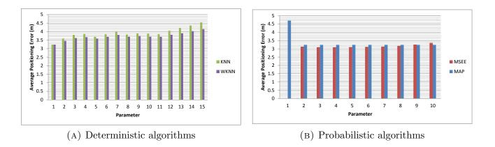
FIGURE 4.45. Average positioning error of the non-dynamic IPS
