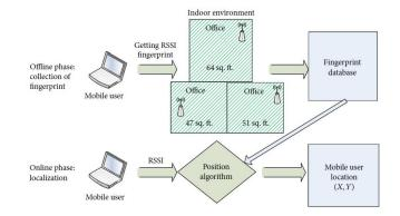
FIGURE 2.7. Positioning using a fingerprinting system
