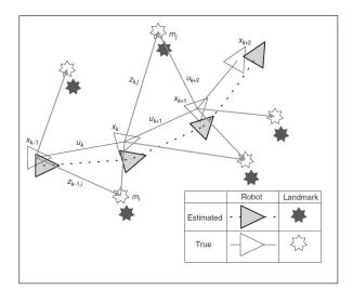
FIGURE 5.1. SLAM using landmarks
