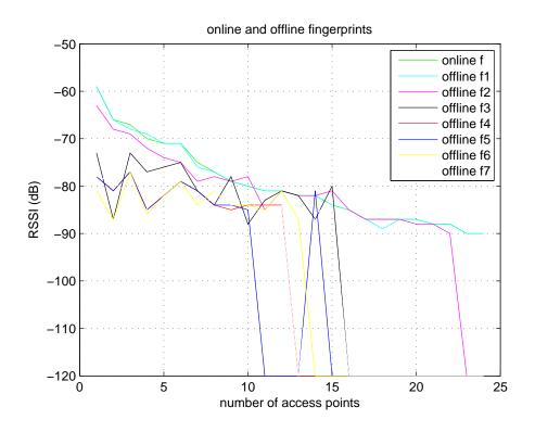
FIGURE 3.3. RSSI levels from 7 fingerprints
