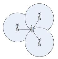
FIGURE 2.8. Calculation of position using TOA
