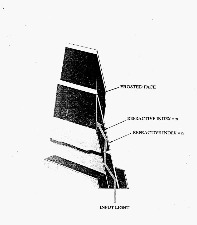
Figure 2 Polyplanar Optic Display Detail
