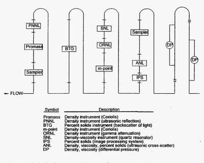
Figure 1. Schematic of pipeline instrumentation test section.
