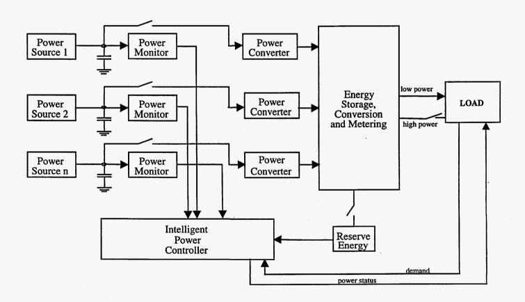
Fig. 1. Concept of power conditioning chip
