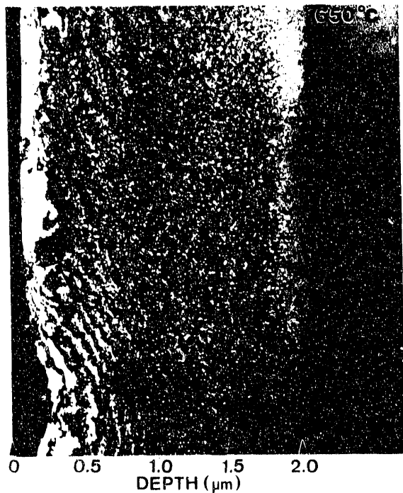
Fig. 1. Cross-section weak-beam micrograph of alumina irradiated with 3-MeV C + ions to a fluence of 5 \times 10^{19} C + /m 2 (0.03 dpa at 0.5 \mu\text{m} ).
