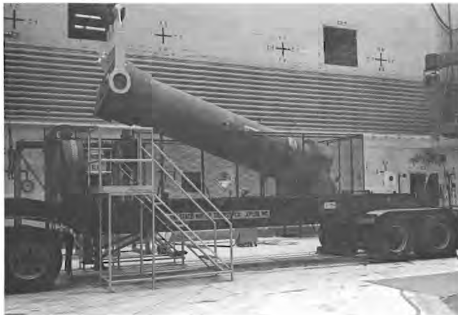
Figure B-24. Spent Fuel Shipping Cask Being Upended in Hot Bay
