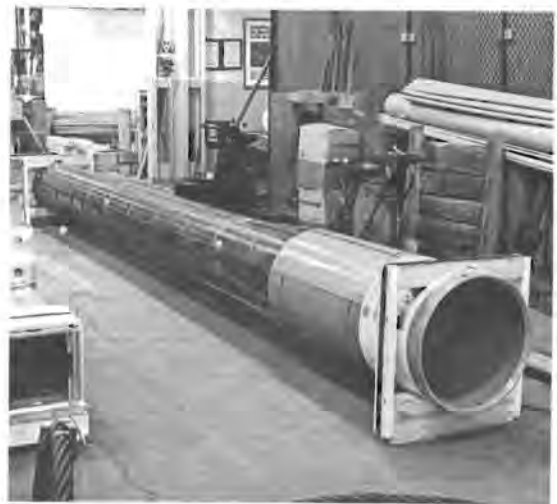
Figure 3.2-17. Drywell Liner Prior to Shipment
