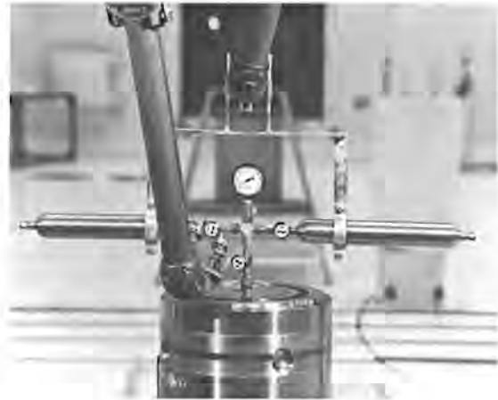
Figure L-2. Photograph of Unwelded Canister Gas Sampling Operation
