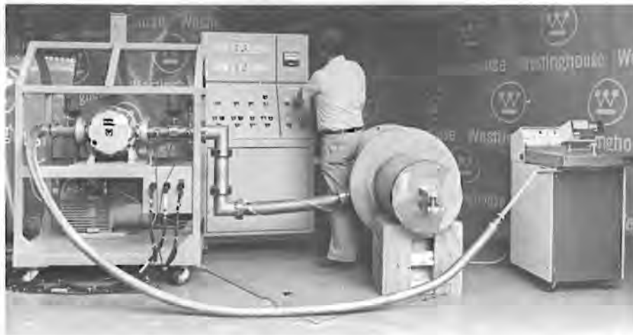
Figure A-21. Canister Leak Detection System Components During Checkout (From Left: Cart Mounted Components, Control Console, Vacuum Chamber, and Helium Leak Detector)
