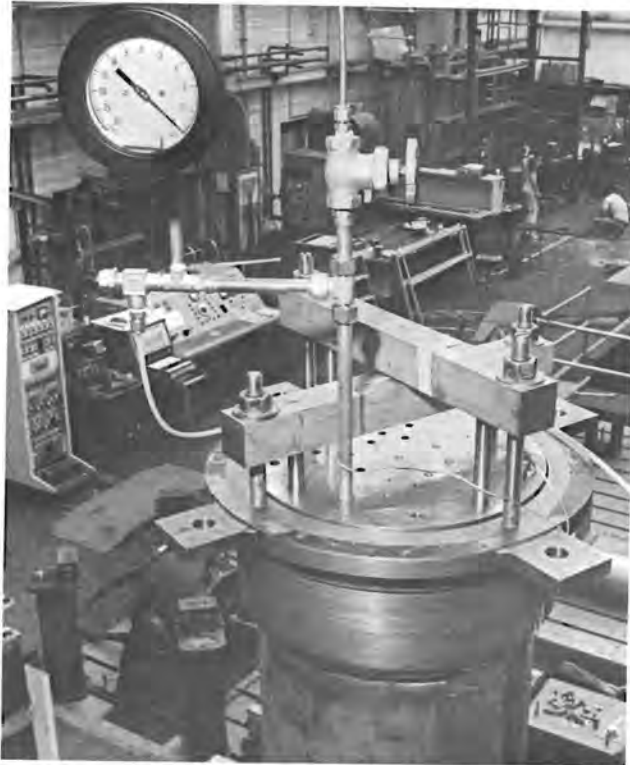
Figure 5.2-10. Test Canister and Closure Lid Assembled for Hydrotest
