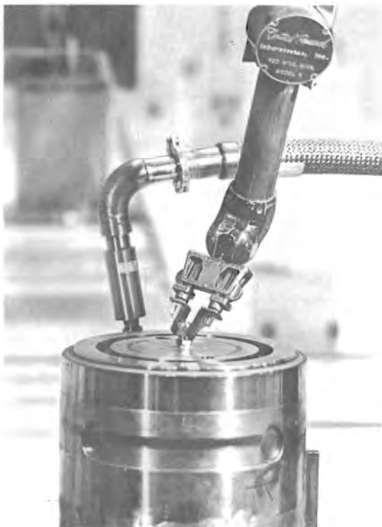
Figure B-45. Installing Closure Lid Seal Fitting After Evacuation and Backfill
