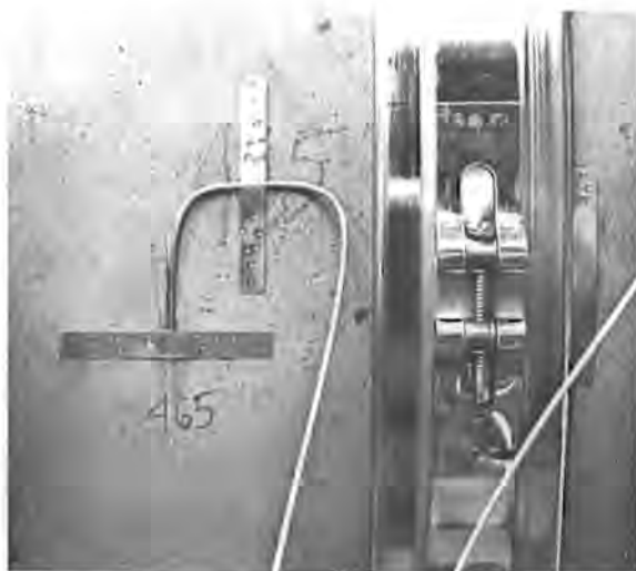
Figure 5.2-6. Liner Heater and Thermocouple Attachment
