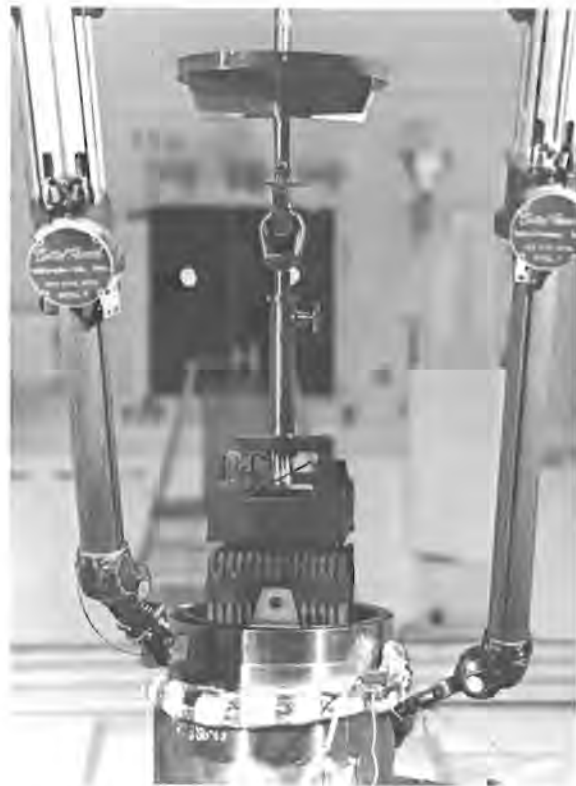
Figure K-2. Fuel Assembly Being Removed From a Canister
