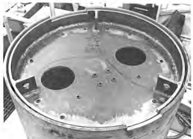
Figure 3.2-9. Top View of Electrically Heated Drywell Test Canister Assembly Shield Plug Fitup Inside Liner
