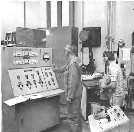
Figure B-48. Leak Detection System Console During Canister Leak Check Operations
