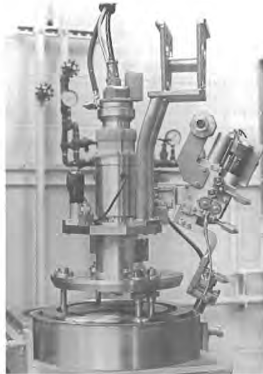
Figure A-17. Canister Closure Lid Welding Machine
