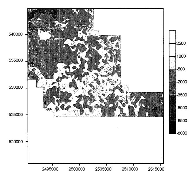
Figure 3–34 Seismic Amplitude of Layton Sandstone, using 110-ft bin data.
