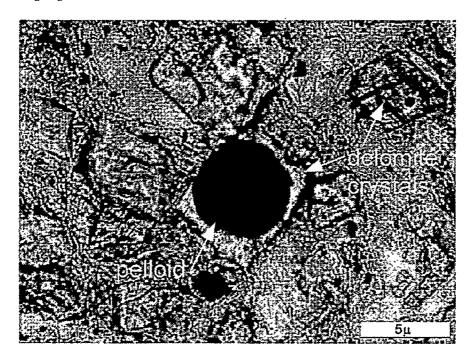
Figure 3–15 Photomicrograph in plan polarized light of coarsely crystalline dolomite nucleating on relict pelloids.
