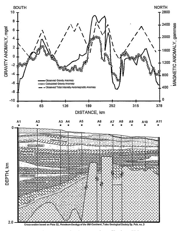
Figure 3–22 Gravity-magnetic profile along SEC1.
