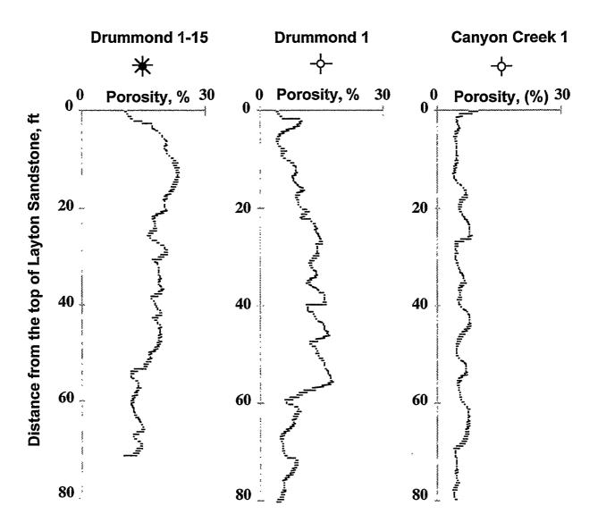
Figure 3–35 Log-Derived Porosity Profiles for Gas-Saturated and Dry Areas.
