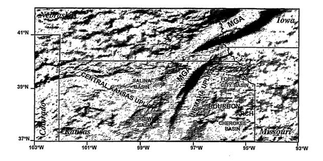
Figure 3-20 Shaded relief map of gravity anomaly in the Mid-Continent region showing major tectonic features. The image is produced by artificial illumination at 135° azimuth and 45° inclination. [MGA - Mid-Continent Geophysical Anomaly].
