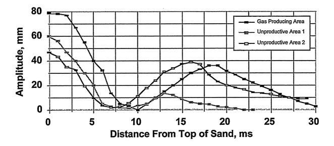
Figure 3–39 Wave Shapes of the Layton Reflector in the Gas-Saturated and Non-Productive Areas.
