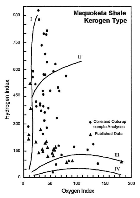
Figure 3–12 Modified Van Krevelen diagram for the Maquoketa Shale. Plotted information is used to determine the kerogen type for potential source rocks.
