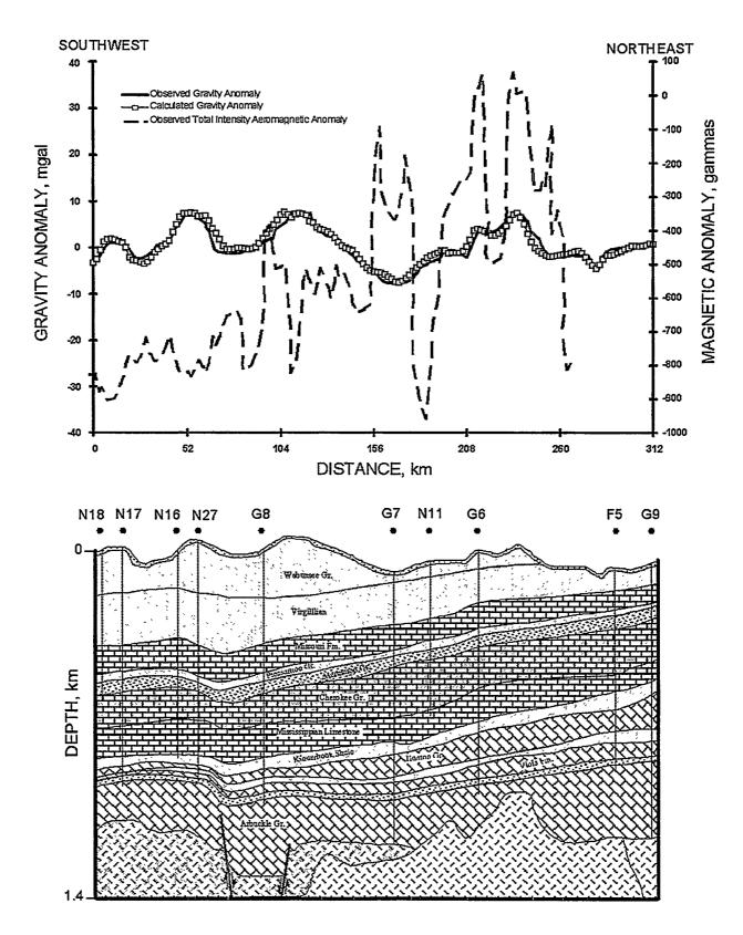
Figure 3–26 Gravity-magnetic profile along SEC 5.
