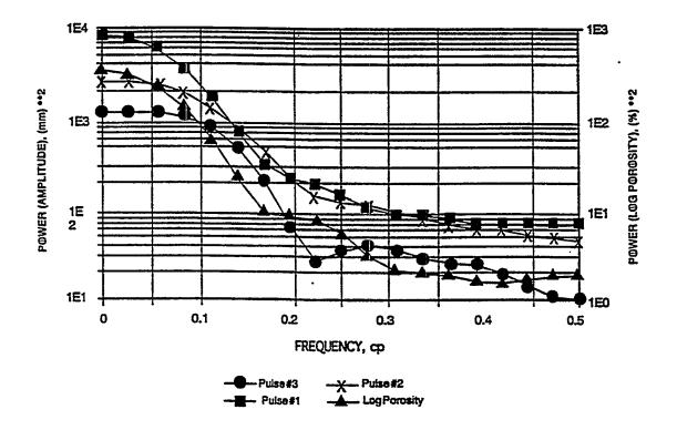
Figure 3–38 Power Spectra of Seismic Amplitudes of Three Seismic Pulses vs. Log Porosity from the Clayey, Non-productive Part of the Layton Sandstone.
