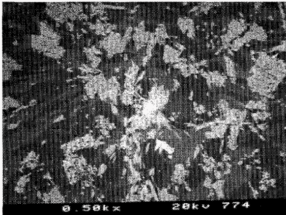
Figure 12. Micrograph (500X) showing predominant phases formed in bottom phase of 127 glass prepared with plutonium oxide.
