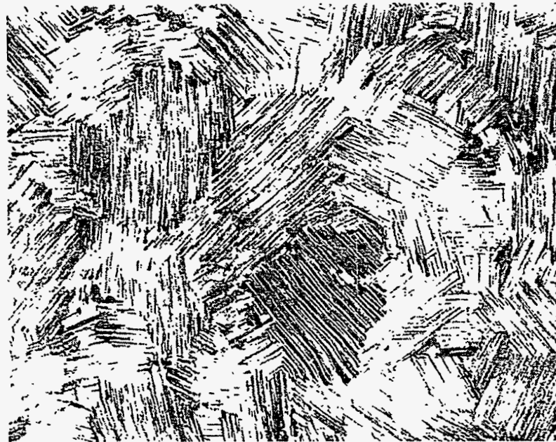
Figure 5. Effect of heat treatment on optical microstructures of cast TIA-27 alloy (a) as-cast, (b) heat treated 20 min/1300°C, (c) 20 min/1320°C, and (d) 20 min/1340°C. 200×.
