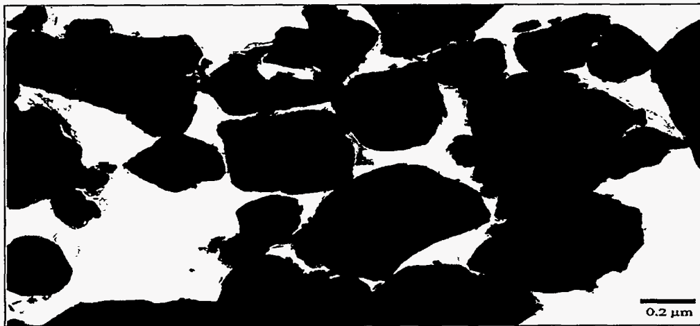
Figure 8. TEM micrograph of WC powder produced from the novel precursors at 1400°C for 2 hrs in flowing 10 % H 2 -Ar atmosphere.
