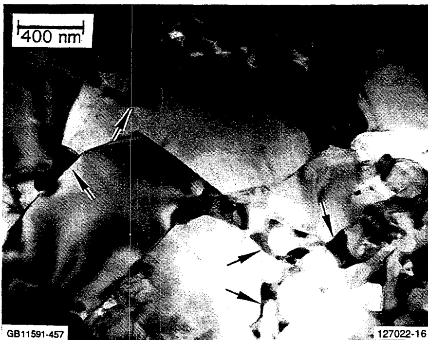
Figure 4-57. TEM Photomicrograph Of NT154 Microstructure, Showing Yttrium-Rich Triple-Junction Crystalline Phases (Arrows).
