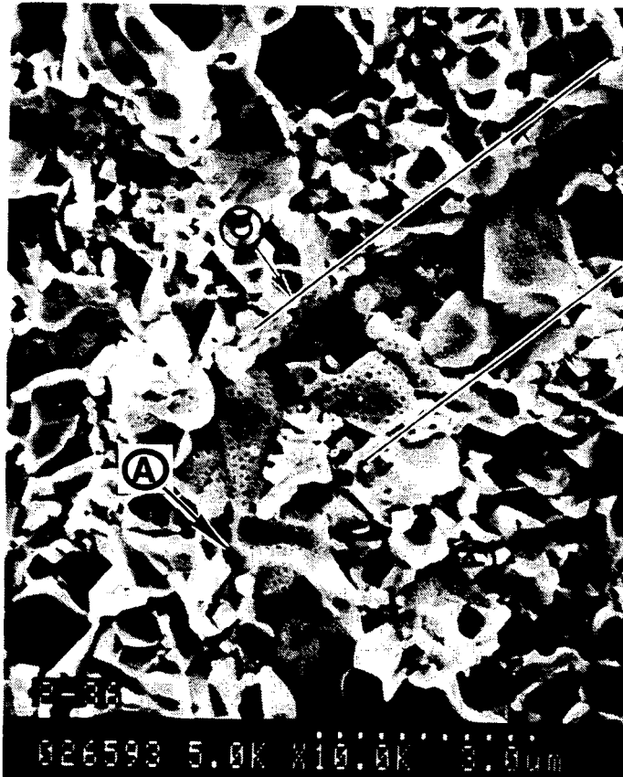
Figure 5-12. Two-Grain Junction Cavitation On An Acicular Grain (A) At 1477K.
