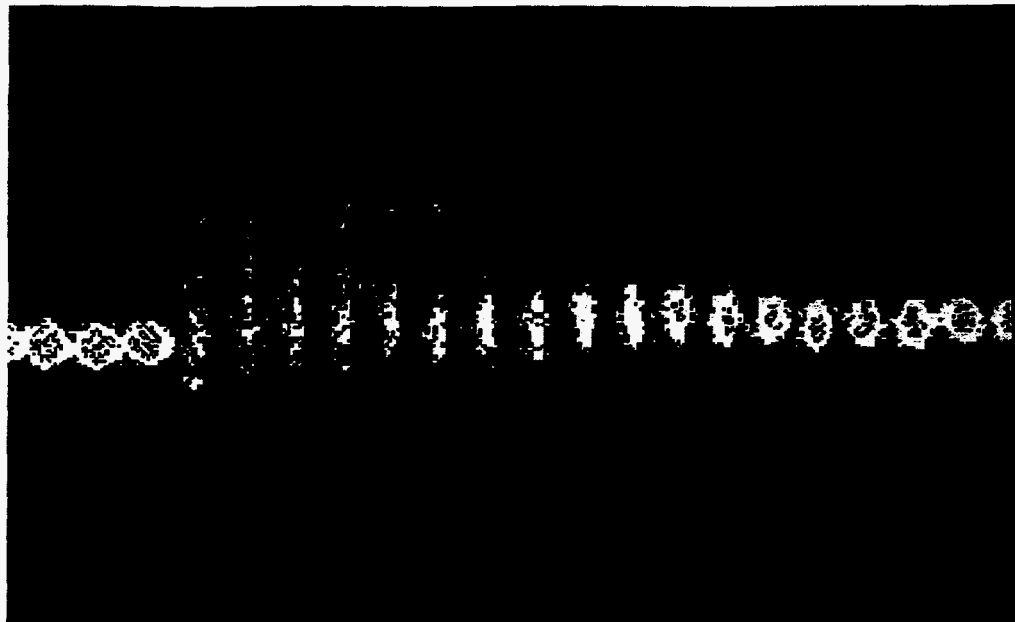
FIGURE 5a. Dual sweep streak image with 12th harmonic turned on. The vertical span of the image is 10 ns and the horizontal is 50 ms. The vertical streak was triggered every 2 ms.
