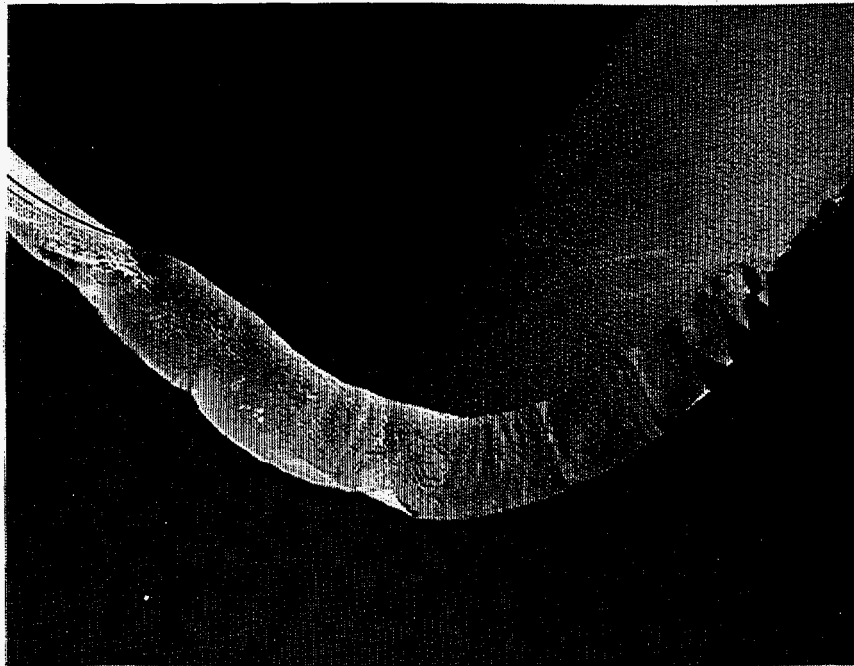
Figure 2.67 Fracture surface from the carbon steel base metal experiment (1.3-2) DRB/1.3-2/F37
