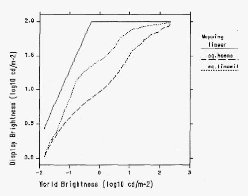
**Figure 13.** The brightness map for the bathroom scene with lights dimmed to 1/100<sup>th</sup> of their original intensity, where human contrast sensitivity makes a difference.
