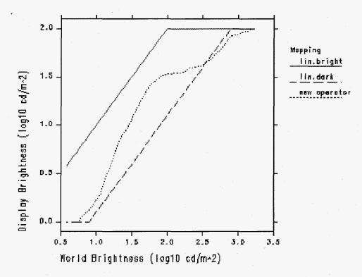
**Figure 7.** A plot comparing the global brightness mapping functions for Figures 1, 2, and 3, respectively.
