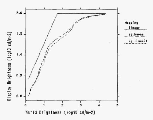
**Figure 12.** Our tone mapping operator based on human contrast sensitivity compared to the histogram adjustment with linear ceiling used in Figure 10. Human contrast sensitivity makes little difference at these light levels.
