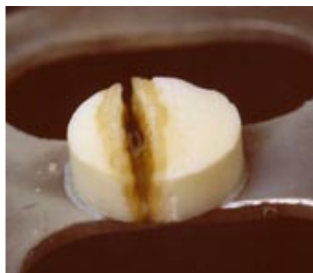
Figure 4. LX-16 cut with a long pulse (.5 ns). Definite signs that a reaction may have occurred are visible.
