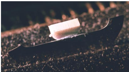
Figure 2. Cross section of an LX-16 pellet. The other half is not shown. The pellet is glued to a stainless steel substrate.
