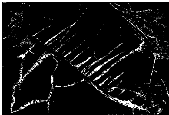
Fig. 4. (Top) 3D volume rendering of crack damage in a triaxially deformed rock (Spruce Pine dunite). The fine crack network in the upper right corner would not be resolvable using conventional LM. The image is 768 \times 512 \times 71 voxels, with an image volume of 430 \times 287 \times 14.4 \text{ μm}^3 . (Bottom) A 2D image slice from the 3D data set. The relationship of the cracks trending NE-SW to the grain boundary (running diagonally NW-SE) is indisputable in the 3D image, but less so in the 2D slice.
