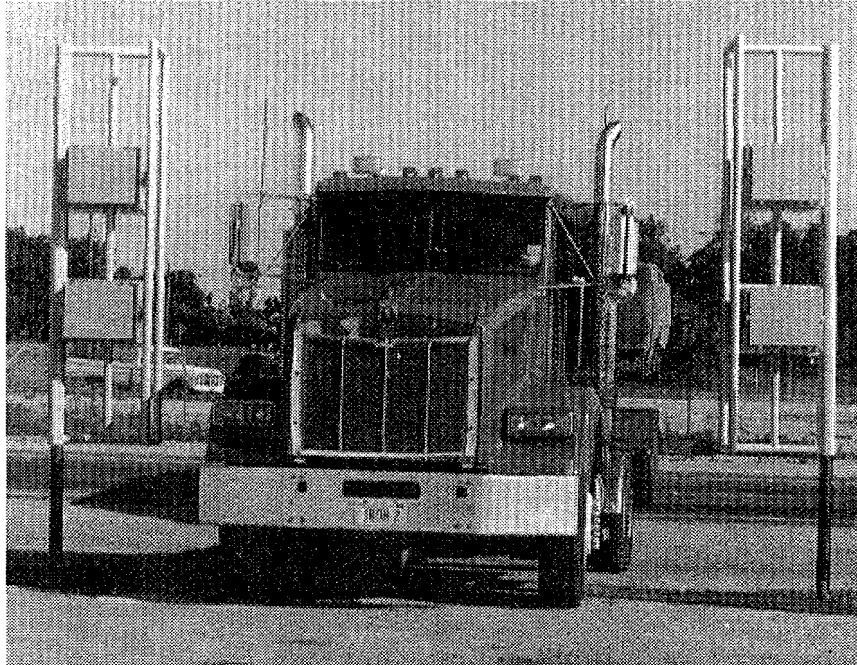
Fig. 6. A simple steel scrap monitor, the Ludlum Measurements, Inc., Model 3500 12 gate monitor.
