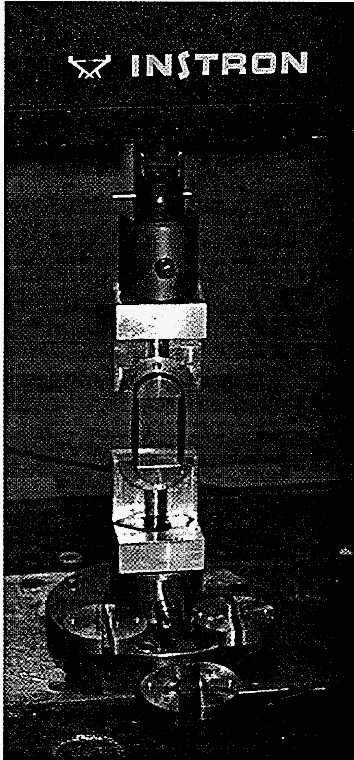
Figure 3. Insert mount and split-spool, interchangeable fixtures for O-ring tensile testing. Insert and split spools fabricated according to Sandia drawings.
