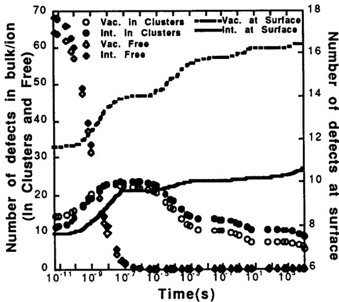
**Figure 4.** Kinetic Monte Carlo results for the annealing of the damage produced by 5 keV Xe implantation at  $1.5 \times 10^{13}$  ions/cm<sup>2</sup>. Number of V and I in clusters and free (left hand side of the plot), as well as the number of defects at the surface (right hand side) as a function of the annealing time. Temperature of annealing is 350°C.
