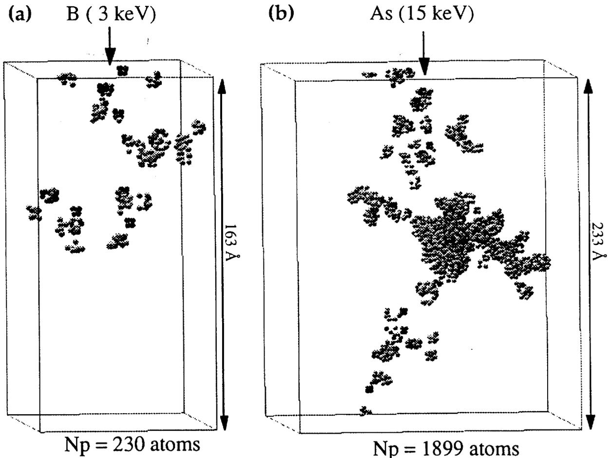
**Figure 1.** Molecular dynamics simulation of ion implantation in Si for (a) 3 keV B irradiation and (b) 15 keV As irradiation. Configuration of atoms with potential energy  $> 0.2$  eV with respect to the ground state, 10 ps after the initial collision.
