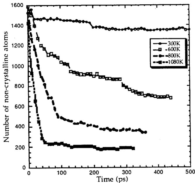
**Figure 2.** Annealing of the damage produced by 15 keV As implantation in Si. Number of non-crystalline atoms as a function of annealing time, for different temperatures.
