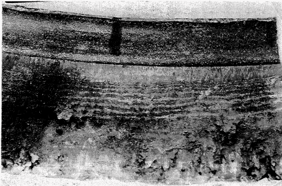
Figure 4.57 5X magnification of the fracture surface for Experiment I-5 at the crack centerline
