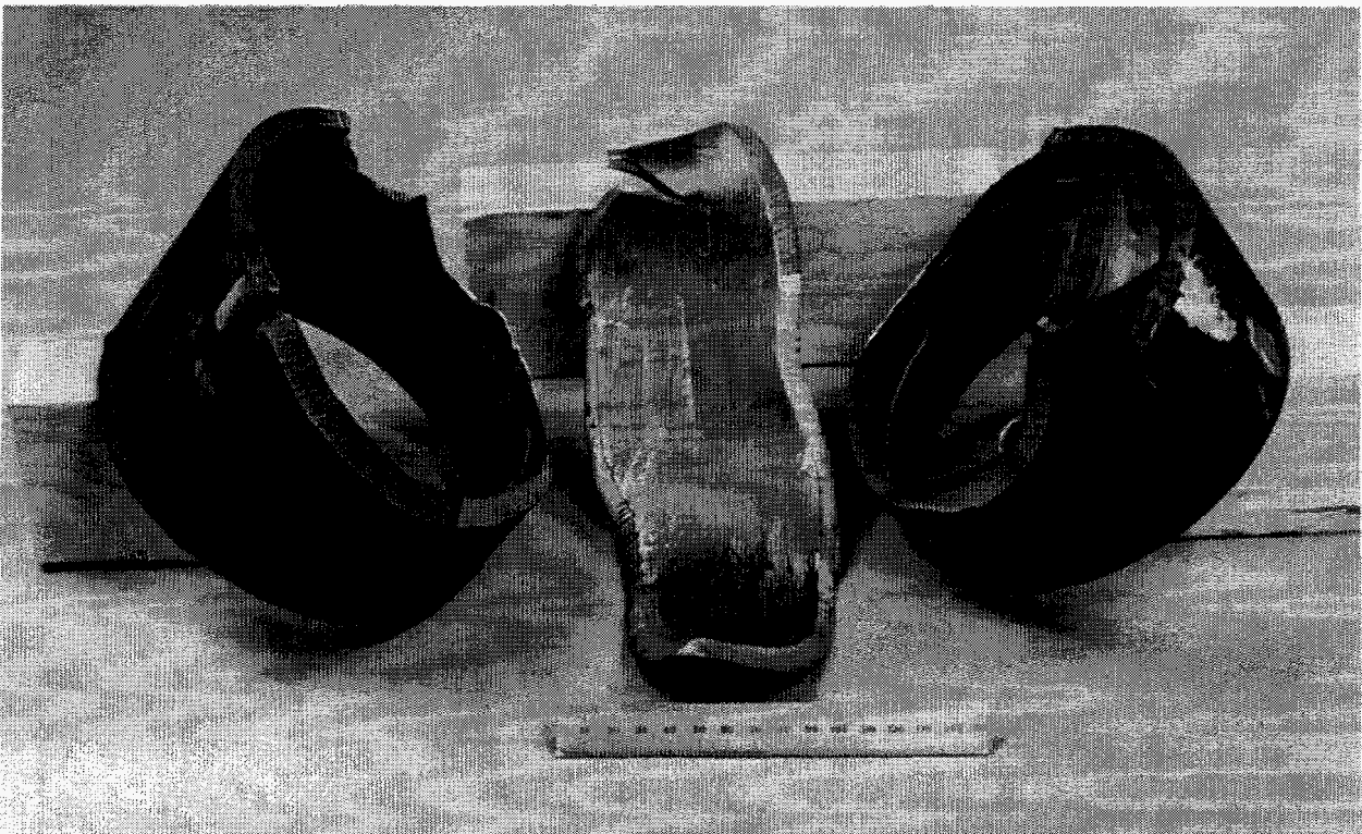
Figure 4.98 Photograph of fracture surface for Experiment 1-9
