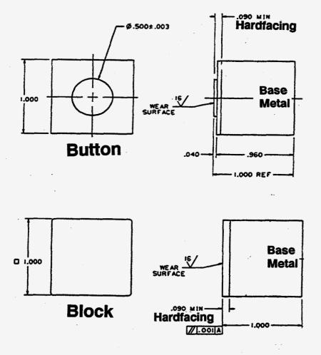
Fig. 1. Schematic of the button and block hardfacing galling specimens.
